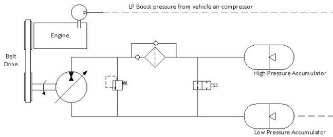
**Figure 6: Hydraulic schematic. Note the low component count, enabled by the Digital Displacement® pump-motor directly control flow and pressure.**
