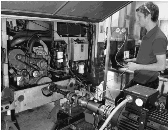
Figure 3: Measuring fuel use with a 30 kw dynamometer connected directly to the crankshaft.
