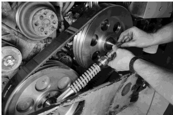
**Figure 7: The belt-drive is spring tensioned to prevent the hybrid system from imposing any additional radial loads on the engine crankshaft.**
