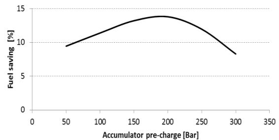
Figure 5: A parameter sweep of accumulator pre-charge pressure to find the optimum.
