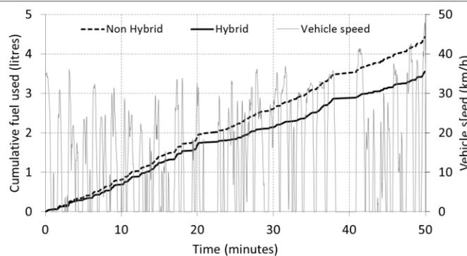
Figure 10: Simulated fuel saving on the MLTB cycle with a conventional automatic transmission and stop-start functionality
