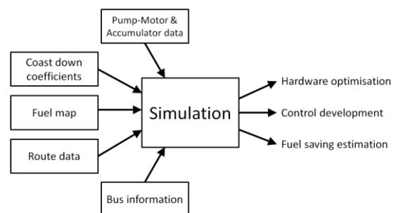
**Figure 2: Input parameters required prior to development of the simulation model**
