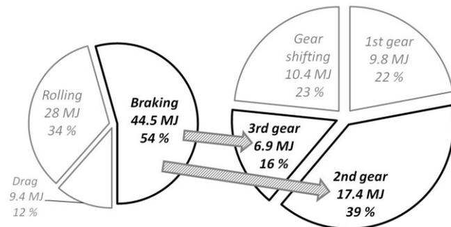
Figure 4: Left: From the measured in-service data, 54% of mechanical energy reaching the wheels ended up as braking energy. Right: 16% of this braking energy was dissipated whilst the bus was in 3<sup>rd</sup> gear and 39% whilst it was in 2<sup>nd</sup> gear. Of the total braking energy, 55% (24.3 MJ) is available to be recovered by the retrofit system.
