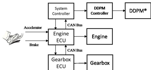
**Figure 9: Communication between hybrid vehicle sub-systems**
