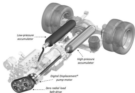
Figure 1: Principal components of the city bus hydraulic hybrid system
