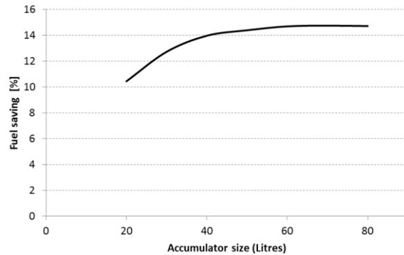
**Figure 8: Accumulator volume optimisation. Diminishing returns are seen above around 40 litres.**
